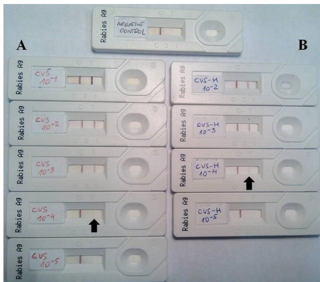
Column (A): serial dilutions in base 10 in the lysis buffer of the kit. Column (B): base 10 serial dilutions, in which the first dilution in PBS was performed. The band of the first dilution is most reinforced in the test line of column A. The arrows indicate the cutting line of both columns.
