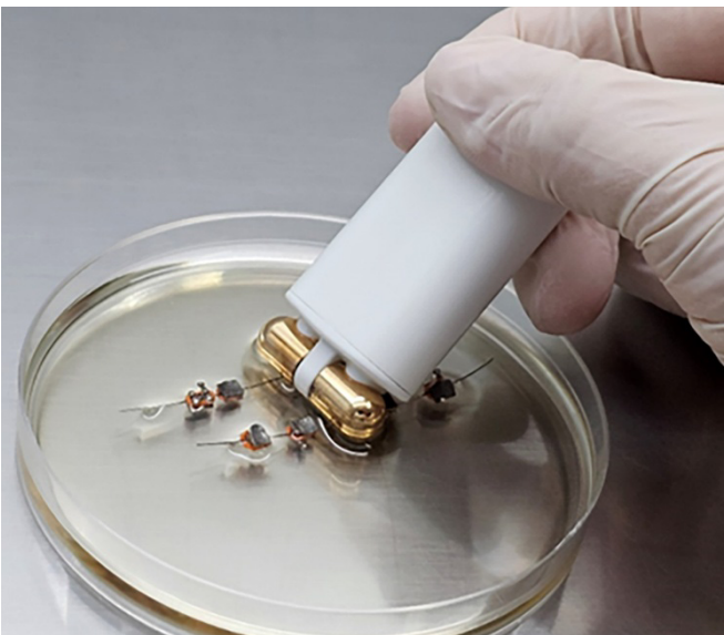
Simultaneous contact with the arch wires of fixed orthodontic appliance (soaked in buffered peptone solution in Petri dish) creates electric field between the wires.
